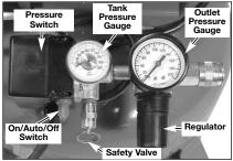
**Safety Valve:** If the pressure switch does not shut off the air compressor at its "cut-out" pressure setting, the safety valve will protect against high pressure by "popping out" at its factory set pressure (slightly higher than the pressure switch "cut-out" setting).
